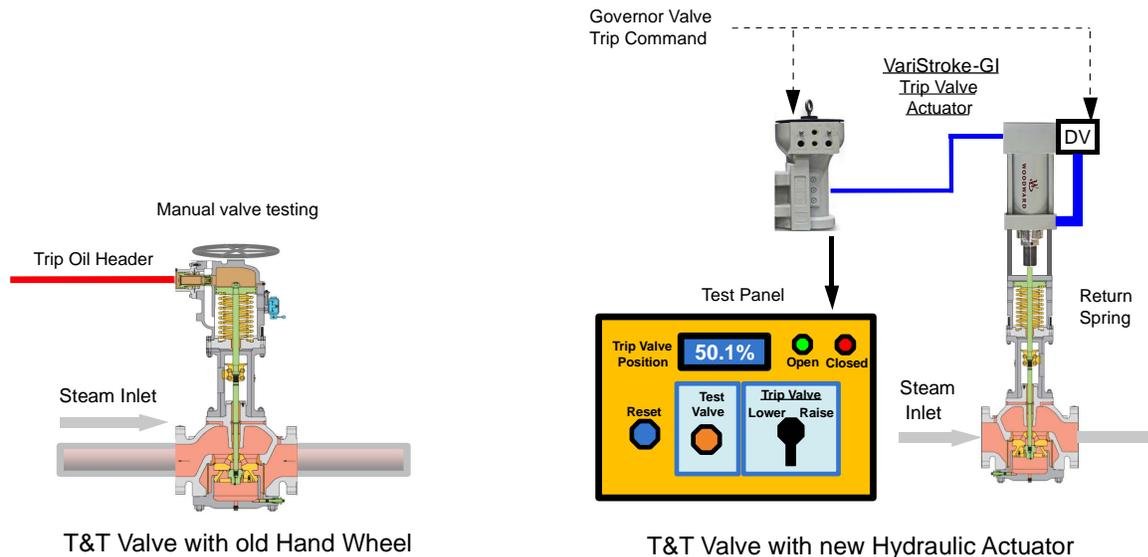
**Figure 1. Example T&TV Hand-Wheel to Hydraulic Actuator Conversion**
