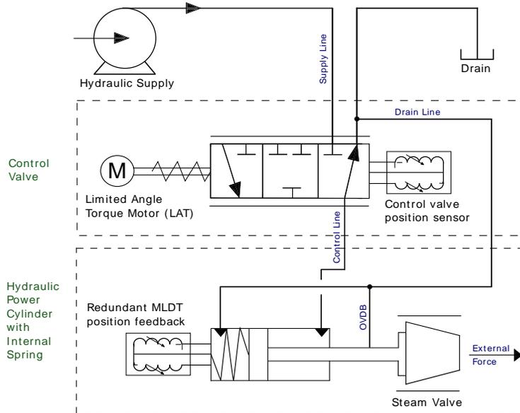
Figure 6. VariStroke-GI Hydraulic Diagram
